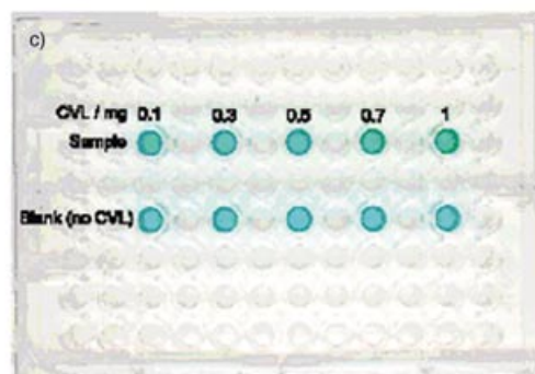
Figure 3. a) Plot of absorbance against time for CVL-catalyzed (varying concentrations) hydrolysis of dimedone ester (R/S)-4 (14 \mu\text{mol} per well) in DMSO/H 2 O/saturated Cu(OAc) 2(aq) (75:15:10, 200 \mu\text{L} per well). b) Plot of the slope versus the amount of CVL per MTP well; c) 96-well microtitre plate (MTP) showing the green colour of adduct 7 .
